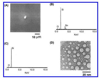
Figure 2. (a) Scanning electron microscope (SEM) image of a  $4 \mu m SnO_2$ dot formed by holding an ink-coated tip on the substrate for 30 s. (b) EDX analysis of the SnO<sub>2</sub> dot. (c) EDX of the SiO<sub>2</sub> substrate outside of the dot. (d) TEM image of the mesoporous SiO2. The image was collected from heated samples with a Hitachi HF-2000 TEM.
