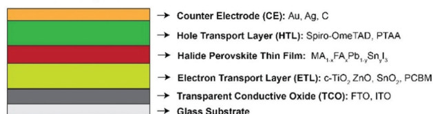
Fig. 9 A simplified schematic of the two main types of PSC architectures that are actively utilized in photovoltaic research. The first type is the meso-superstructured solar cell (Top) and the other is the planar, thin-film solar cell (Bottom). The heterojunction of both devices can be configured between the regular (n-i-p) or the inverted (p-i-n) archetypes, with respective material changes to HTL and ETL.
